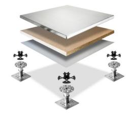
This product illustration shows the main elements of the panel (particle board encapsulated in galvanised steel sheet) and supporting pedestals<sup>1</sup>
