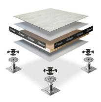
This product illustration shows the main elements of the panel (particle board with top & bottom galvanised steel sheets plus vinyl finish) and supporting pedestals<sup>1</sup>
